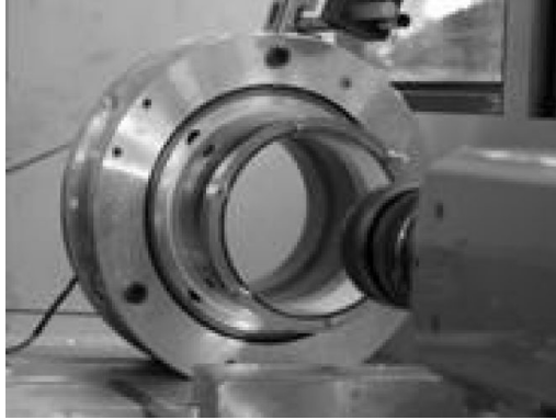
FIGURE 2. Picture of the experimental device showing the tank. In the front is the high-speed camera. At the back the toothed belt can be seen.
